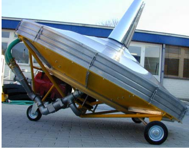
Figure 5. Moteur Stirling solaire sans concentration SUNPULSE [8]
